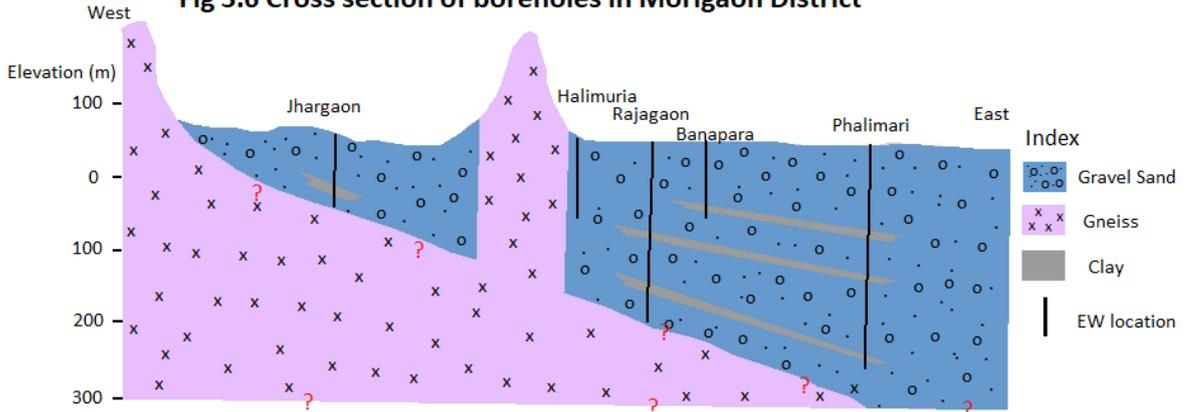
**Fig 3.7 Cross section of boreholes in Morigaon District**
