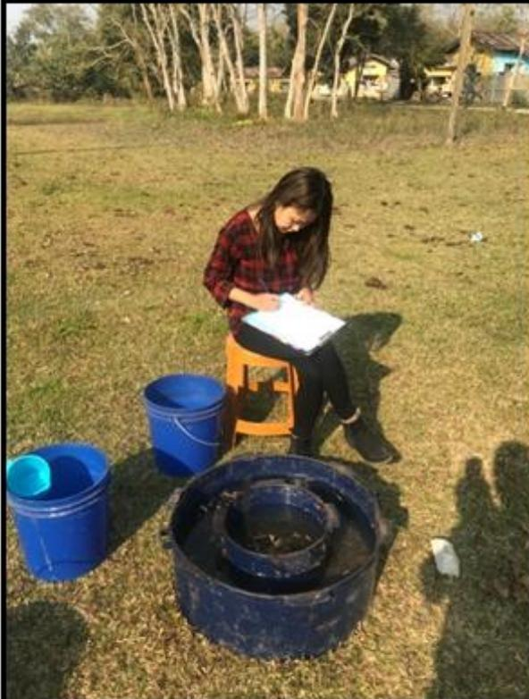
**Soil infiltration test**
